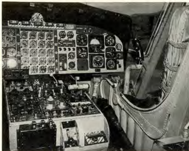
Control stick is a stick, not a yoke. Note collective power lever between pedestal and seat.
