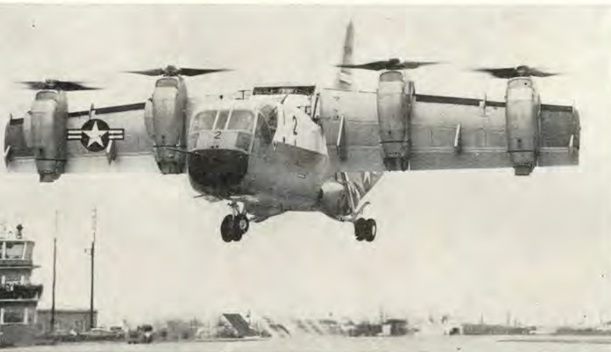
Straight up! Props are interconnected, if one engine should fail others will drive that propeller by means of cross-shafting. Aircraft cruises on two engines turning all four props.
